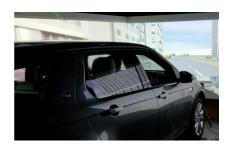
The Southampton University Driving Simulator (SUDS), which currently comprises a Land Rover Discovery vehicle and Triumph motorbike linked to the STISM Drive M500W – Wide Field-of-View System with Comprehensive Vehicle Dynamics Model and Active Steering.
